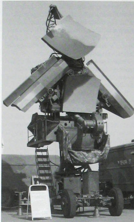
> This Pechora-2T radar is fitted with Tetraedr's new electro-optical sensors.
