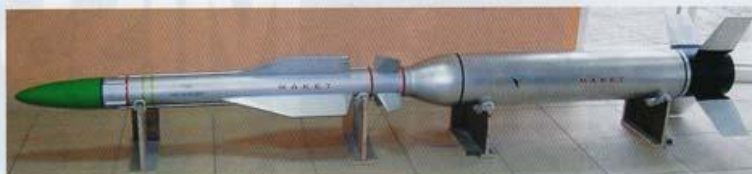
This mock-up shows the planned configuration of the Luch T382 two-stage missile. This will replace the older single-stage missile used by the Osa system and offers twice the range and twice the maximum engagement altitude.
