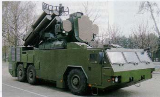
Despite the change of chassis, the T381 combat vehicle of the T38 Stilet system shows its Osa lineage, but eight ready-to-fire rounds in circular container/launchers replace the six-round armament of the original version. Tetraedr: 1331559
