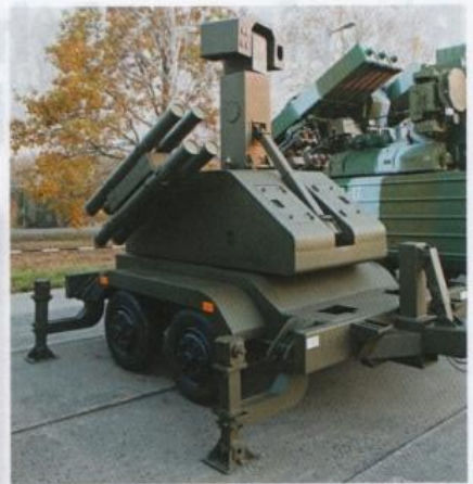
The first customer for the A3 system chose to have the combat module – seen here armed with anti-tank and manportable air defence system (MANPADS) missiles – mounted on a wheeled trailer. Miroslav Gyürösi: 1331265
