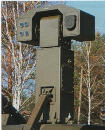
The combat module's mast-mounted electro-optical unit is based on the OES-1T sensor unit that the company developed for its upgraded Osa-1T self-propelled surface-to-air missile system. Miroslav Gyürösi: 1331267
