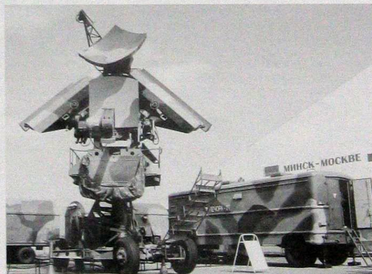
> The UNV fire-control radar seen here is a derivative of the original SNR-125 ('Low Blow') radar. The associated equipment cabin is seen at the right.
